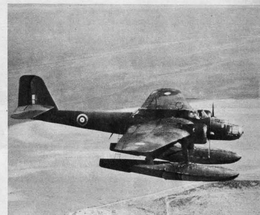
Long nose, twin floats and the wing's tapered leading edge help distinguish the He-115. It was the first Nazi plane to sow magnetic mines.
